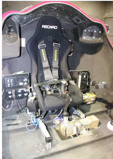
(a) CMS with closed cabin mounted on linear axis. (b) Inside view of cabin with controls.
