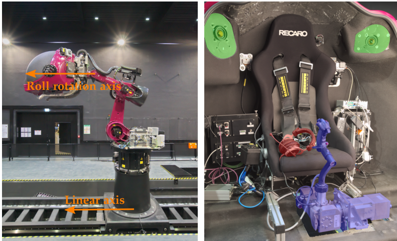
(a) CyberMotion Simulator (CMS) in position to start next experimental trial. The orange arrows show the roll rotation axis and the linear axis. (b) Cabin of the CMS with cyclic control stick (blue), projection system (green), and the communication headset (red).
