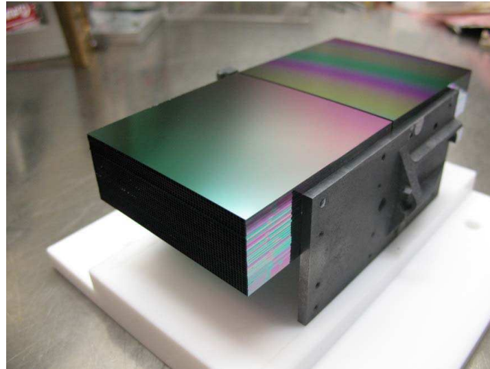
Figure 2.9.: a) shows the functional principle of a single pore of an SPO. These pores are formed through stacking multiple groove cut wafers. By aligning two of these wafer stacks, a single mirror module is formed. Each pore is a small sector of a Wolter-I telescope. Multiple mirror modules are assembled into a mechanical frame to form the complete ATHENA mirror system as shown in figure 2.10.
