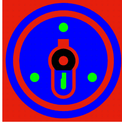
Figure 4.25.: Layout of a Blindgate Pixel. The color code is equal to figure 4.3a. The red areas mark p+-implantations as drain, source and the surrounding drift-ring. The n+-implantations of blind and clear are marked in green, while the blue areas are the clear-gate and blind-gate contacts, implemented in the first poly-silicon-layer. The black donut-shape is the external gate, implemented in the second poly-silicon layer.
