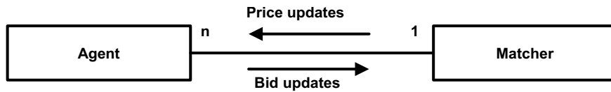
Figure 5.1: Generic agent roles in PM: agent and matcher. Agents express bids to a matcher based on the flexibility in supply and demand they represent. The matcher determines the price for its agents based on the supply and demands bids.
