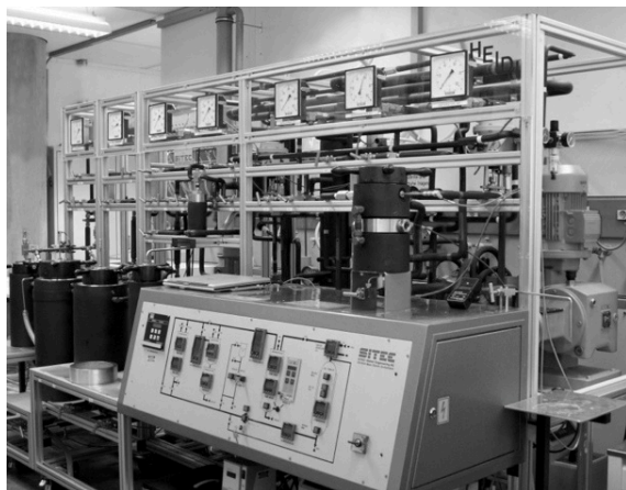
Figure 8 Pilot unit used for high pressure micronization
