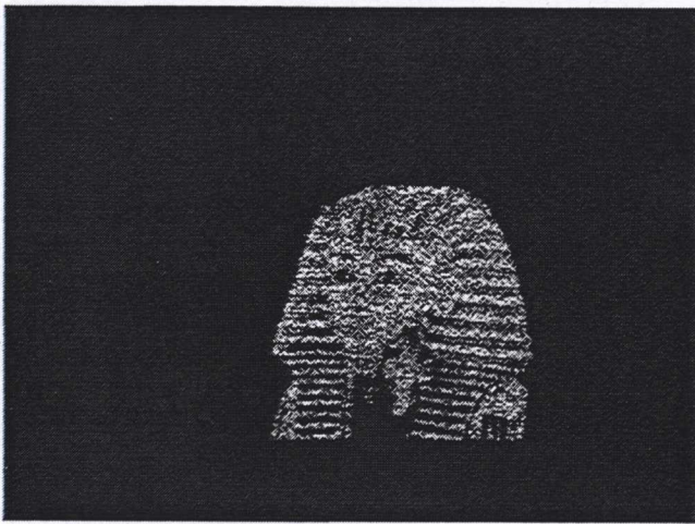
Figure 2.17b: Foreground image, separated at grey level 111.
