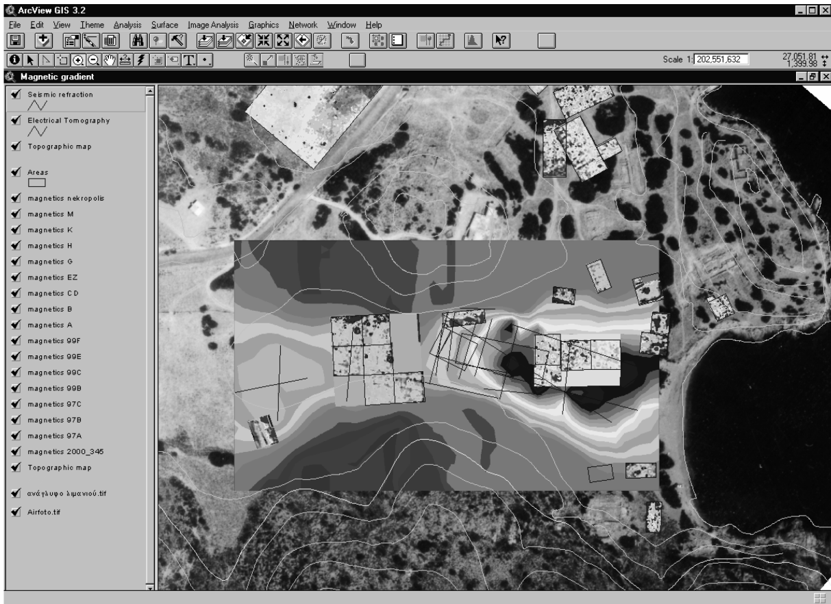
Fig. 1. A typical geophysical data presentation in GIS. The georeferenced datasets from the ancient port in Itanos are listed to the left. The magnetic gradient map consists of several small subgrids (dark grey denotes high values). The large image corresponds to the bedrock relief (black denotes low elevation). Elevation contours in white exhibit 4 m contour spacing. The aerial photograph is displayed in the background.
