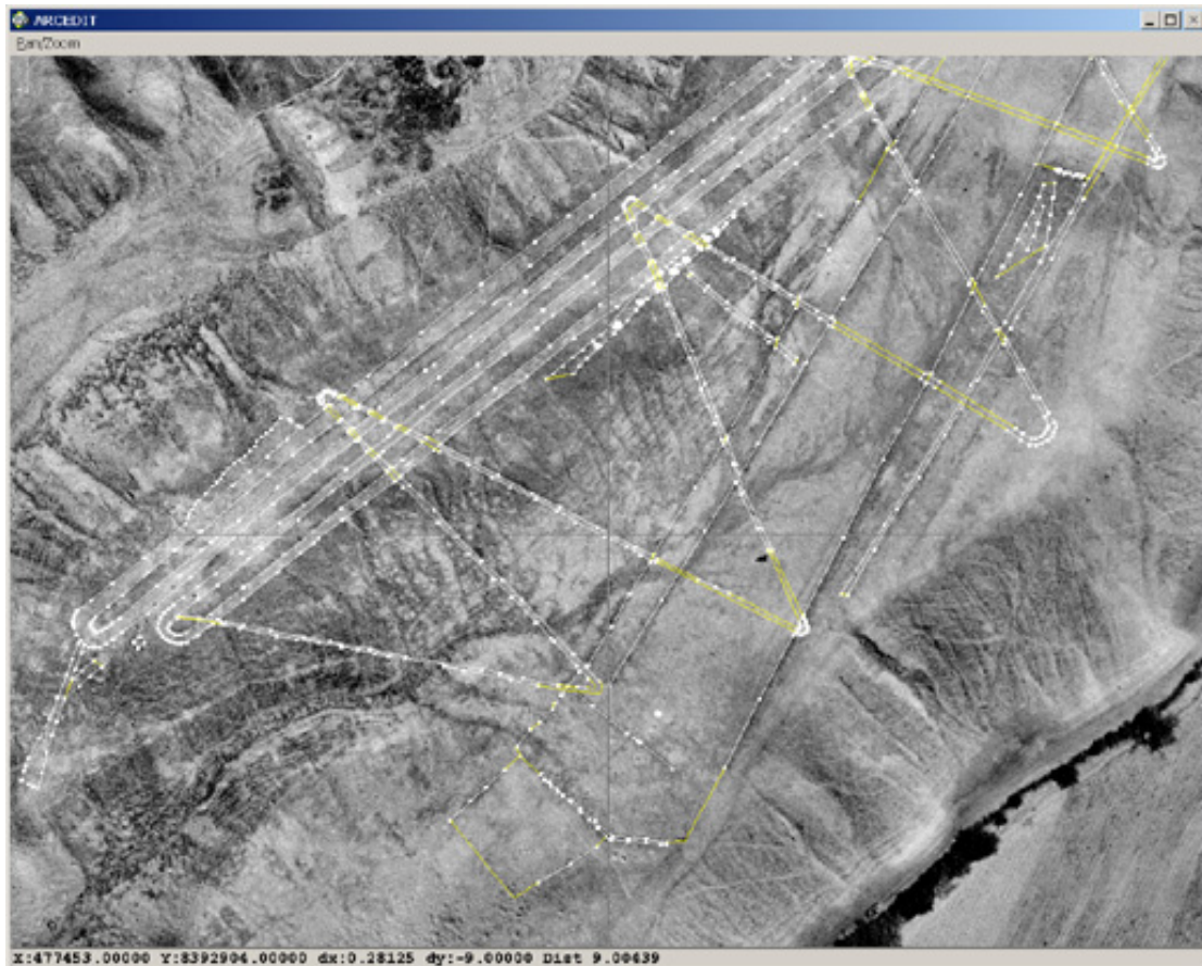
Figure 3 – ArcGIS/ArcEditor user interface showing the orthoimage as background layer and the completed sections (yellow) of the measured vectors (white)
