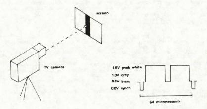
Figure 1: Brightness waveforms for a simple scene.
