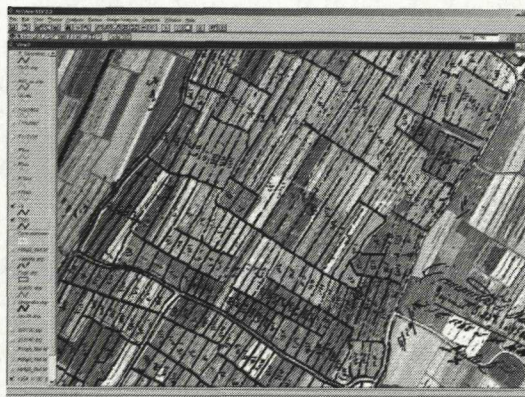
Figure 1 The vectorialisation of cadastral map overlaid on the aerial photo of 1954. A detail of Sesto Fiorentino Plane
