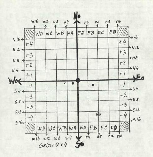
EXAMPLE: If the find is at the exact intersection of £6 and S2, the measurement should be taken from the intersection of E4 and S-Zero.
