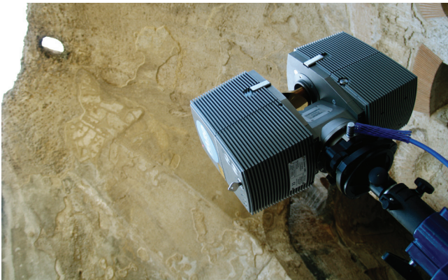
Fig. 2. 3D digital survey: laser scanner (FARO 80.80) is working under the Serapeo's large vault.
