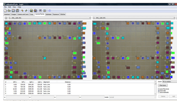
Figure 2. Lens calibration calculation within Hugin using a tiled wall surface as the target.
