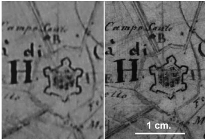
Fig. 1. Comparison of detail between images obtained by photographic (on the left) and direct scanning (on the right) procedures.
