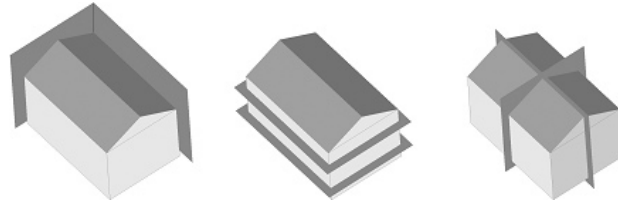
Fig. 4. 2D descriptions derived from 3D data sets: Façade views, floor plans and intersections.
