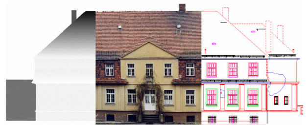
Fig. 7. Digital surface model (DSM), digital orthophoto (DOP) and vector data.
