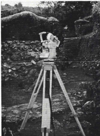
Figure 3. The Wild T1010™ theodolite with a Leica Distomat™ Laser EDM. Photo by Joseph Nigro.
