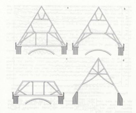
Figure 1: Lincoln Cathedral St. Hugh's Choir roof. (a) truss with tie beam (b) truss with bearers (c) half truss (d) truss adjacent to tower
