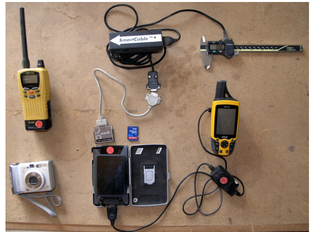
Fig. 1. Each team's equipment. From top, clockwise, SmartCable SPC to serial interface, Mitutoyo digital calipers, Garmin GPS, GPS charging and communications cable, HP iPAQ, Canon digital camera, Navcom RT-250 radio, Socket serial to CF card adapter, and a memory card.
