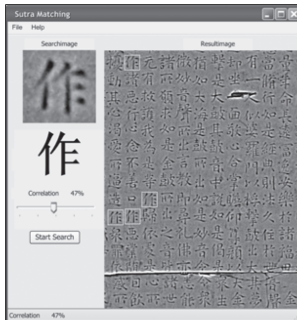
Figure 7. Automatic identification and localization of character in the images using template matching.
