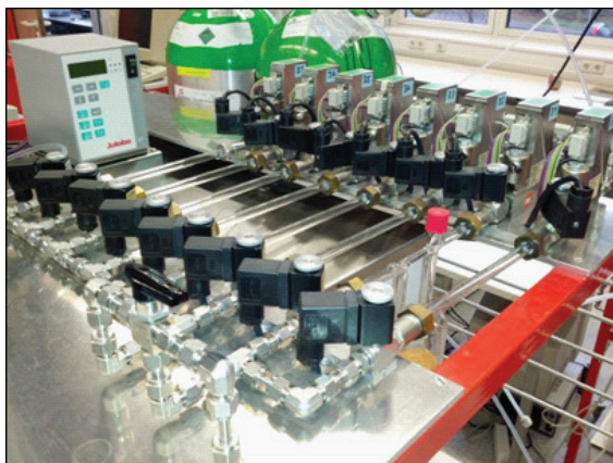
Figure 4.10: Gas mixing system used in the laboratory at the University of Tuebingen
