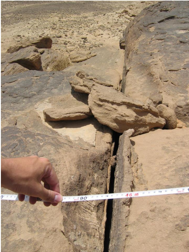
Fig. 9 Typical fracture in the sandstones of the Upper Wajid at Al Jufrah
