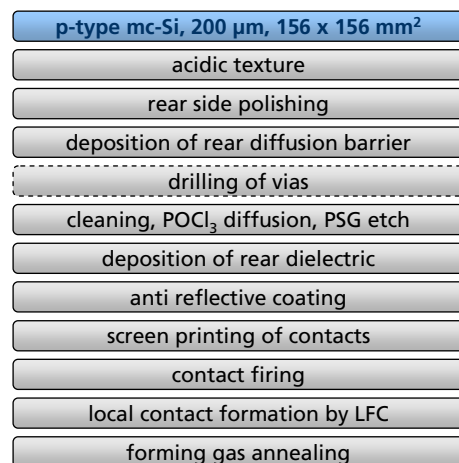
Figure 2: Process sequence for the fabrication of the presented mc-Si HIP-MWT solar cells. Laser drilling of vias (dashed border) forms the only additional process step compared to a typical PERC-type process sequence.
