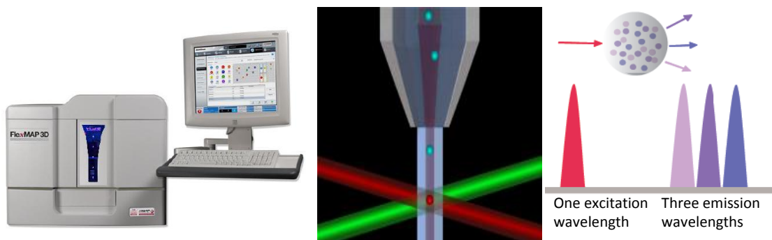
Figure 1-4: Luminex xMAP technology. Adapted from [82]
