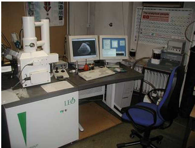
Figure 8: SEM - Laboratory: The SEM (model Leo - 1450VP) at the Institute of Geosciences, Tübingen
