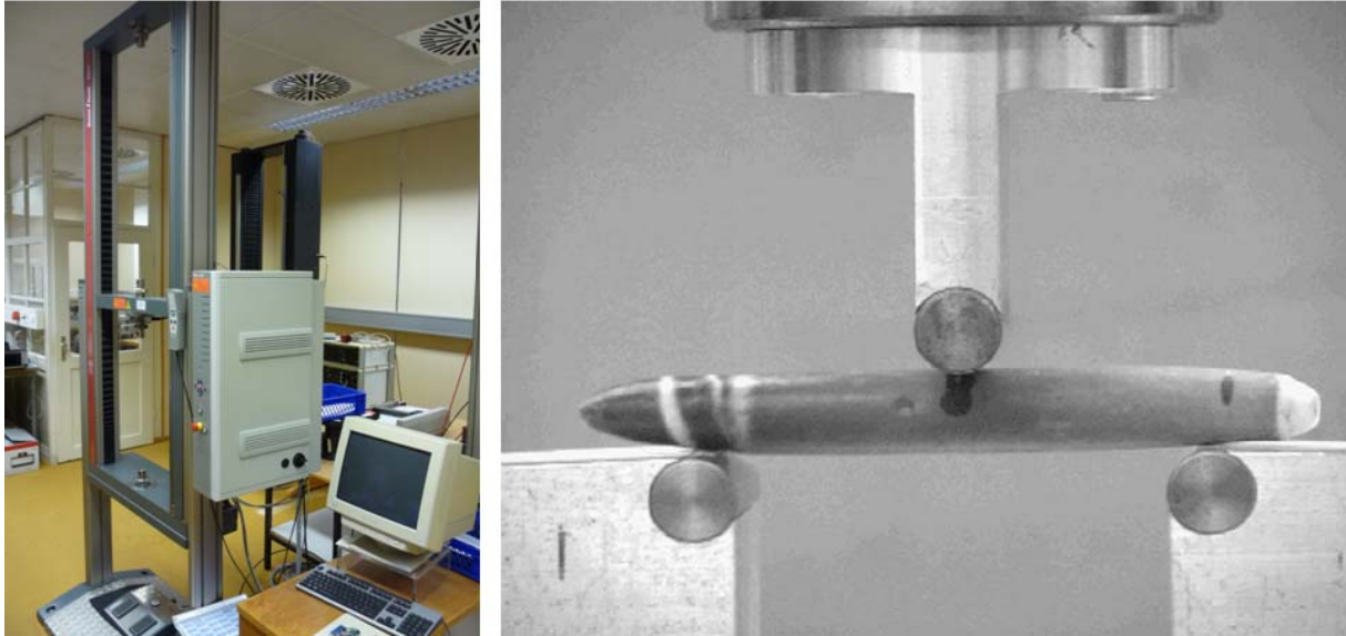
Figure 3: The Zwick material testing machine at the Institute of textile and process engineering (ITV) (left) and a detailed view during a 3-point-bending-test
