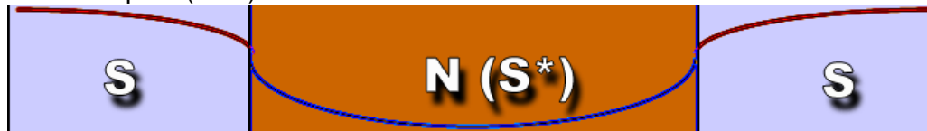
Figure 4.23: Superconducting proximity effect. A superconducting material (S) is in contact with a normal conducting material (N) or a superconductor with a smaller band gap (S*). The superconducting wave function of S (in red) reaches into the N/S* part (blue).
