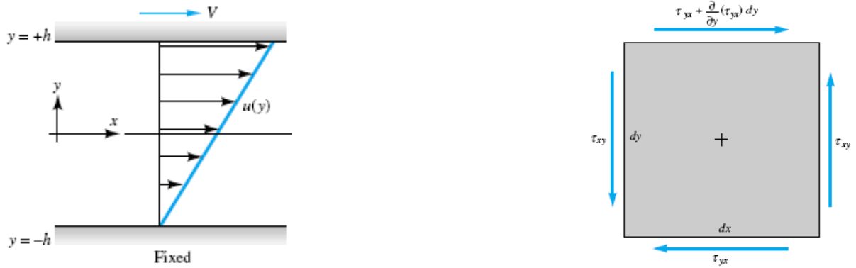
Figure 2.1.1: Shear flow between two parallel plates (left) and forces on a fluid element (right), see [78]. ( x = x_1 , y = x_2 )
