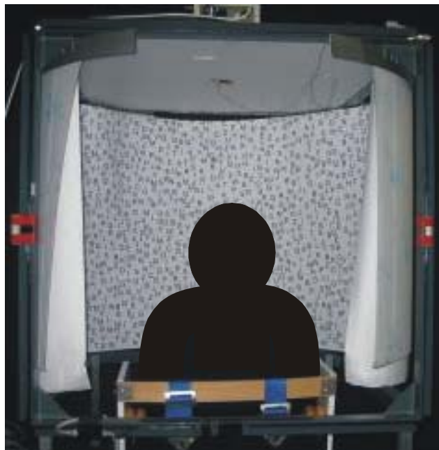
Figure 8. Magnetic search coil system to measure gaze and head-on-trunk positions. Three orthogonal alternating magnetic fields were generated by three pairs of Helmholtz coils mounted on the outer surface of a cubic frame (diameter 105 cm). Patients sit centrally and can move the head freely while the trunk is immobilised by a belt and shoulder straps. On the inner surface of the frame, a unitary array of black letters on a white ground is presented that covers a rectangular area of \pm 120^\circ left and right of the mid-sagittal plane, and of \pm 40^\circ above and below the eye level. The room can be normally lightened or completely darkened, depending on the experimental condition (cf. Procedure).
