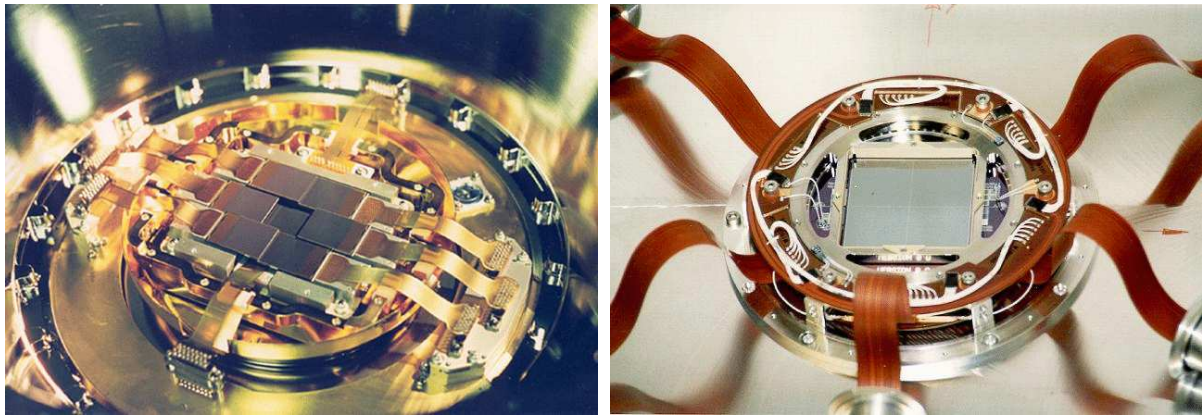
Figure 3.2: The focal planes of the MOS- (left) and pn-camera (right) on board of the XMM-Newton observatory. MOS: image courtesy of Leicester University, University of Birmingham, CEA Service d'Astrophysique Saclay and ESA; pn-camera: image courtesy of MPI-semiconductor laboratory, MPE, Astronomisches Institut Tübingen and ESA
