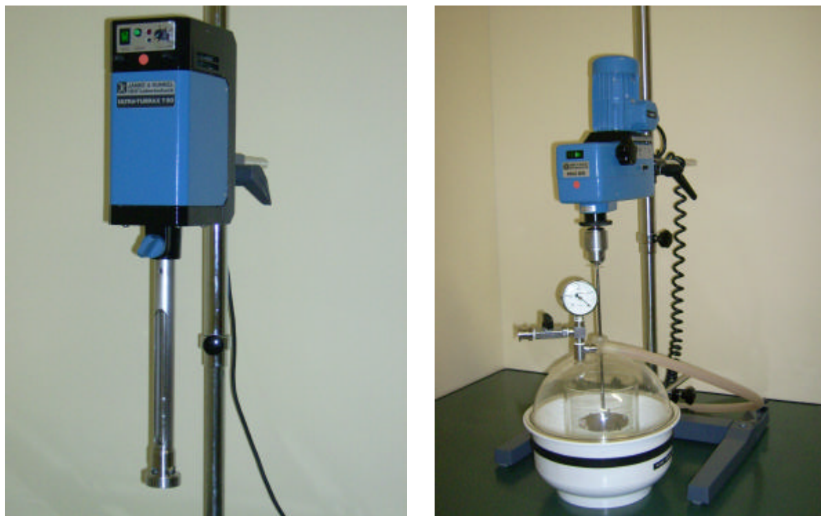
Figure 2-5: Ultraturrax T50 (left), Lab mixer RW 25 (right)
