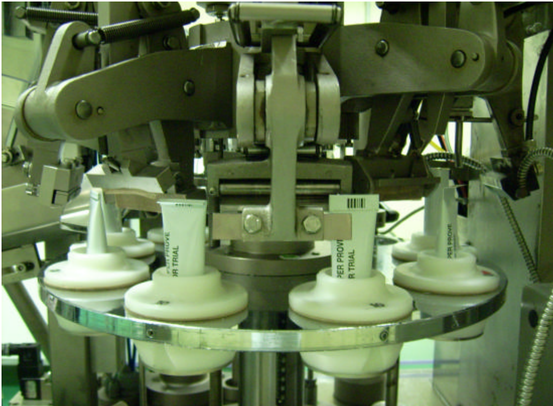
Figure 2-13: Filling process (a); Sealing, folding and imprint (b)
