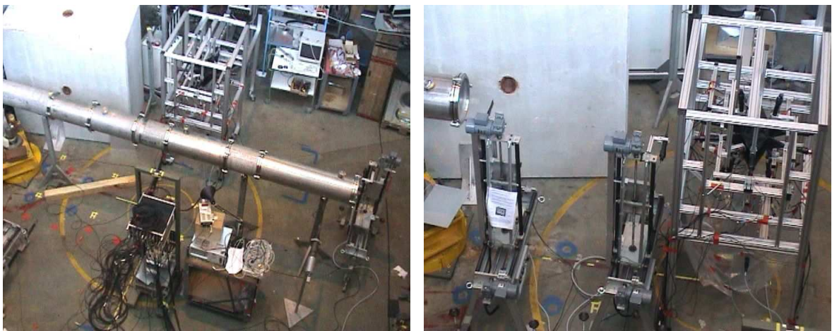
Figure 4.6: Experimental area of the \pi M1 beam line: With the 4\pi detector setup (right) and with the setup for the beam line calibration (left) where the detector was replaced by a 6 m vacuum extension pipe
