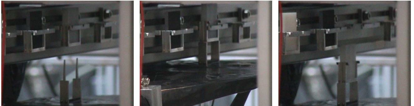
Figure 4.10: Insertion of the thick CH_2 -target during a measurement
