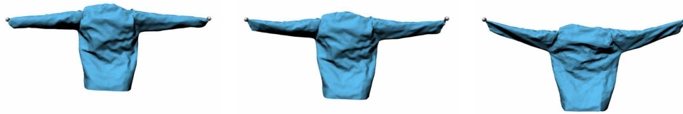
Figure 3.3: A shirt consisting of 31,046 vertices is pinned at two points and dragged down by gravity.
