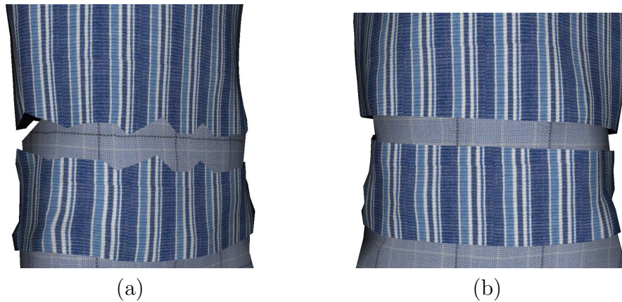
Figure 5.21: A pullover is shortened by cutting a piece off. Image (a) shows the cut without aligning the vertices along the cut edges. In (b) the vertex positions have been corrected and a straight cut is obtained. All the modifications are automatically transferred to the planar patterns.
