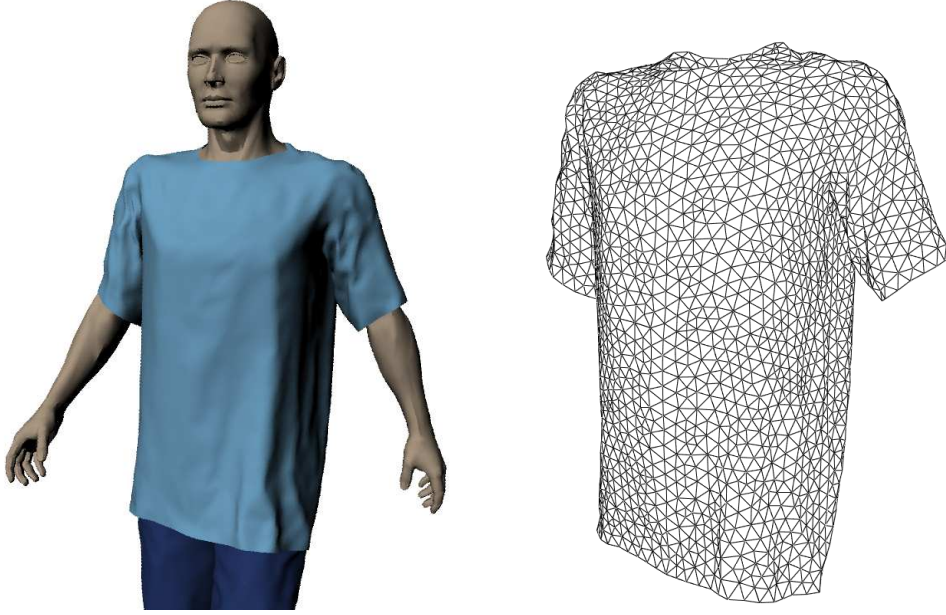
Figure 1.1: Textiles are discretized by polygonal meshes. The shirt on the left is represented by an unstructured triangle mesh, shown on the right.
