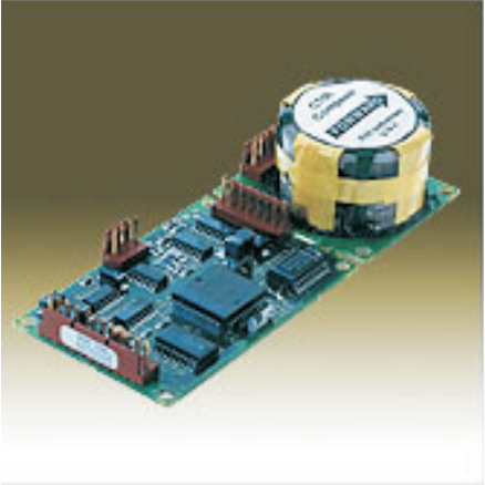
(b) KVH C-100 fluxgate compass
