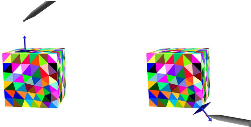
Figure 5.42: A collision proxy plane separates the haptic point from the deformable object. For smooth regions (left) plane normal and surface normal coincide, for sharp features, the closest distance vector used as plane normal shows its benefit.
