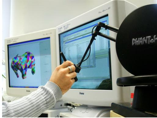
Figure 5.40: Using the phantom to manipulate a deformable model.
