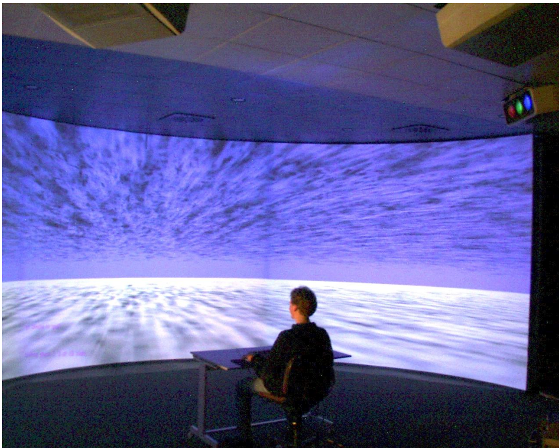
Figure 1: Virtual environments lab with 180 degree projection screen displaying the 3D field of blobs. The participant is seated behind the table in the center of the half-cylindrical screen. On the table are mouse and keyboard as input devices.
