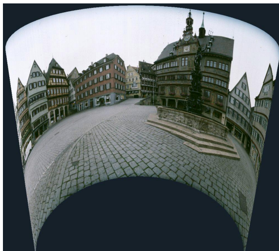
(a) Photorealistic model of the Tübingen market place, created by wrapping a 360^\circ roundshot photograph onto a cylinder. This creates an undistorted view for the observer positioned in the center of the cylinder.
