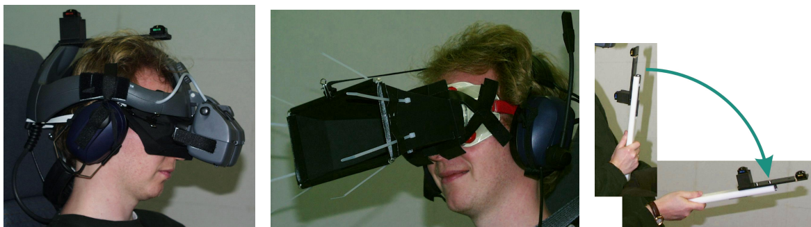
(a) Participant wearing position-tracked head-mounted display ( 40^\circ \times 30^\circ FOV, 1024x768 pixel) and active noise cancellation headphones.
