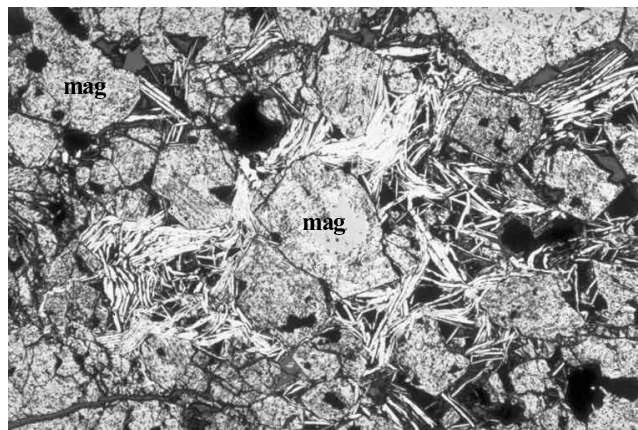
Figure 3.26: Partly ductile deformed as well as broken lamellar specularite between magnetite crystals from the Terra Nera deposit (long side 1100 \mu\text{m} ).
