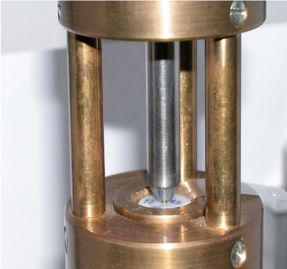
Fig. 5.3. Picture of the apparatus for the biaxial flexure strength test.
