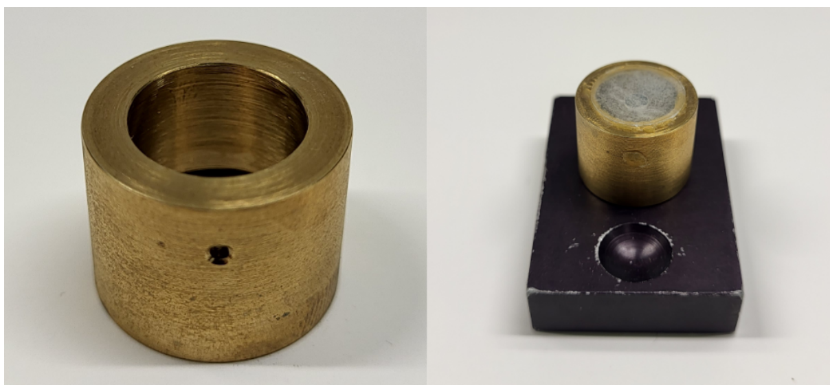
Figure S14. Images of the brass inert chamber attachment (left) and the fully assembled setup (right), including the sample holder, KBr window, and sealing grease.
