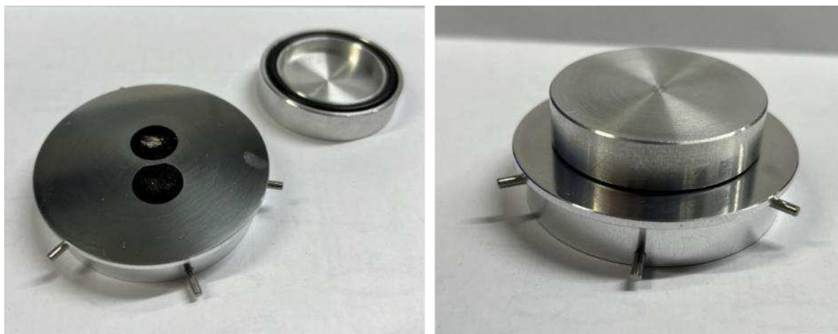
Figure S4. Sample holder and lid for inert transfer for XPS measurements. The sample is fixed onto the sample holder using carbon tape (left). The lid is placed on top of the sample holder, evacuated within the glovebox airlock, and then rapidly flooded with argon to ensure airtight seal (right).
