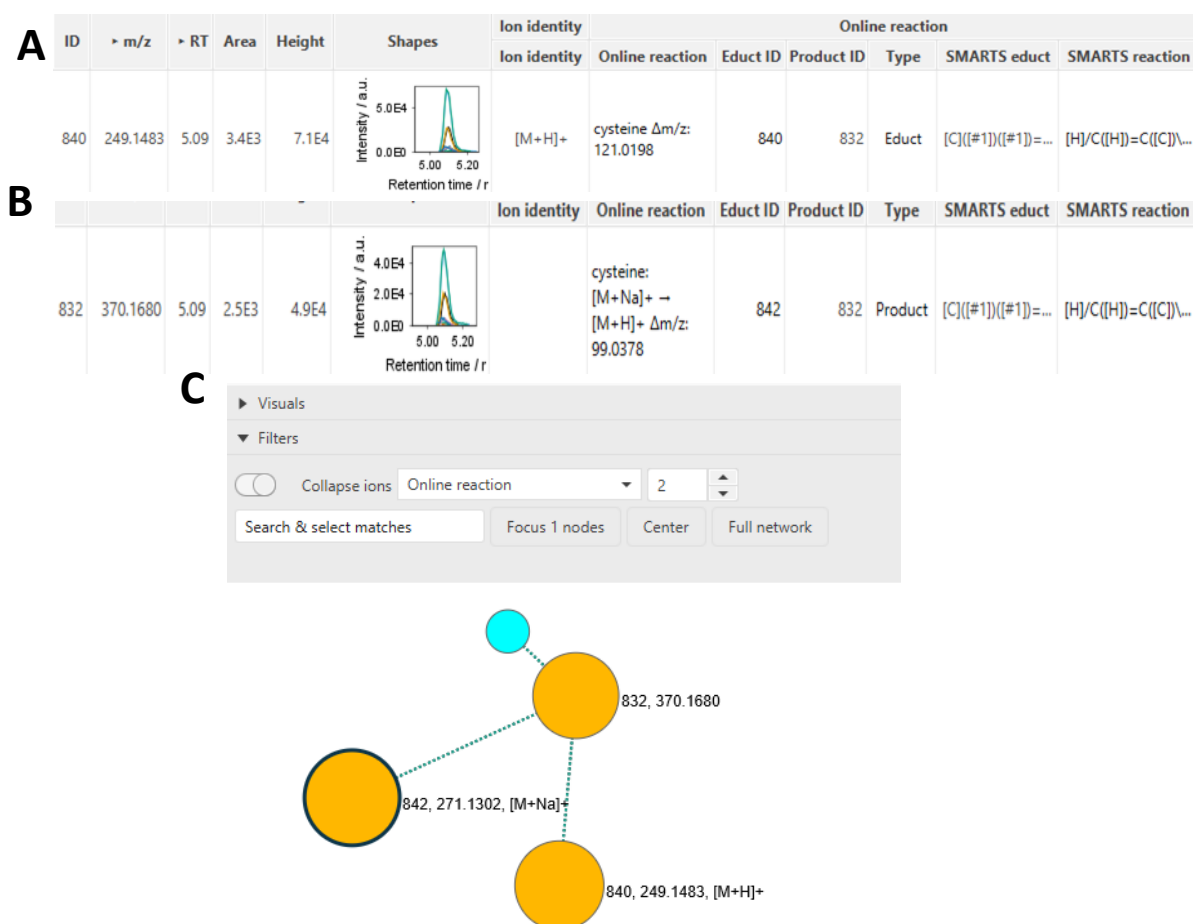
Figure A 42. Features visualization in Mzmine 4 Online Reactivity. In the feature list, it is possible to activate the visualization of the online reaction attributes, such as the observed online reaction (including the ions involved) with the respective \Delta m/z , educt, and product IDs, the status of the feature we are observing (educt or product) the putative educt substructure or the entire reaction (in the form of SMARTS). Here are shown as an example A) parthenolide [M+H] + ion row and B) parthenolide derivatization product [M+H] + with cysteine row, automatically connected by the Online reactivity module. By clicking on the feature, it is possible to visualize the relative networks where the cyan node represents the reaction product. C) Reactivity network of parthenolide.
