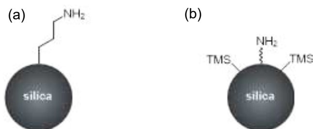
Fig. S20. Surface chemistries of (a) classical APS and (b) polymeric APS according to manufacturers.
