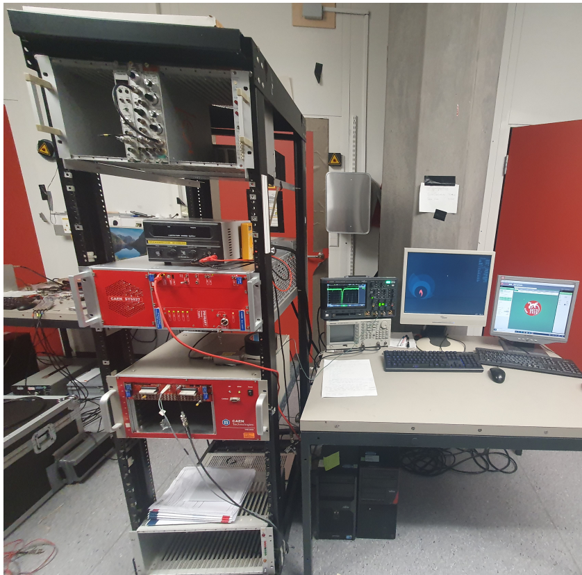
Figure D.1.: Picture of the PMT test stand DAQ electronics. The rack houses the power supplies for the LED , the tested PMT , and the ADC . On the table, the DAQ PC is positioned next to the oscilloscope and frequency generator. A second PC controls the voltages of the PMT power supply, since the operating system of the DAQ PC does not support the power supply software.
