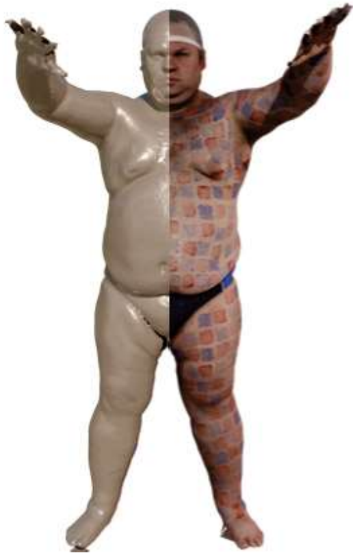
Figure 2.6: Mesh output by a 3D scanner. The left part of the image shows the mesh without texture.
