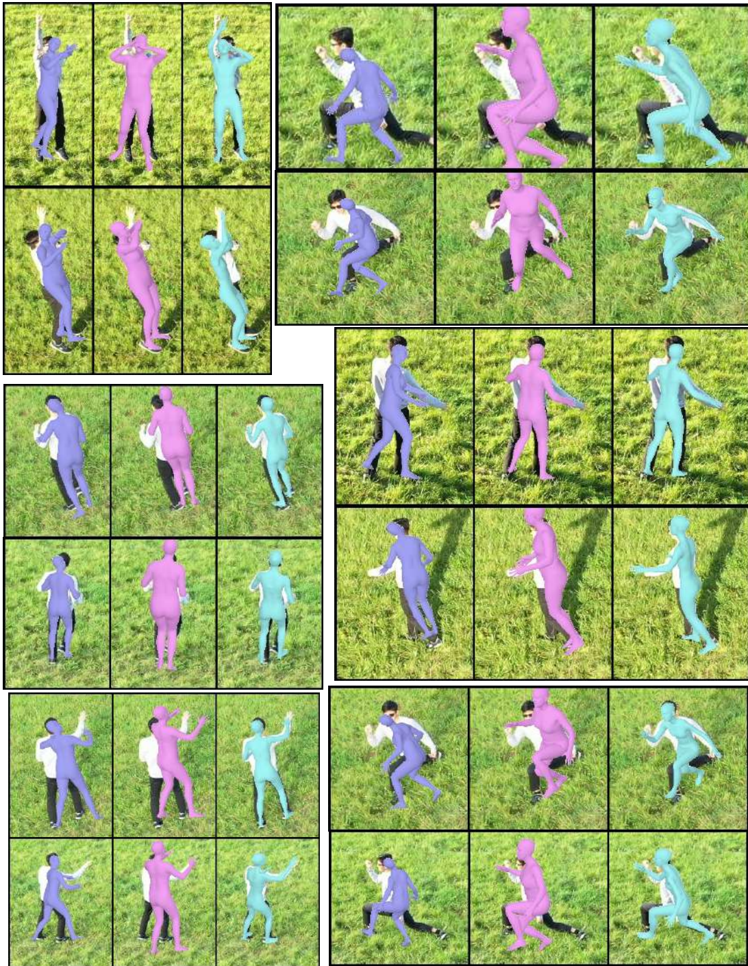
Figure 3.9: Real data. Baseline, AirPose and AirPose + results on real data samples. Each sample contains a 2x3 grid of images with the estimated mesh overlaid. Each row corresponds to one camera view and each column shows projected results from the baseline (blue), AirPose (pink) and AirPose + (cyan).
