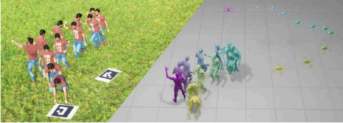
Figure 3.1: AirPose: A novel, distributed, multiview fusion method for 3D pose and shape estimation of humans using uncalibrated moving cameras. Multi-exposure image of a sequence from our real-world data (left). AirPose + estimates of the person (right). UAV poses are also estimated but here we manually place them for clearer illustration. ArUco (6) markers were in the scene but never used for any of our methods.
