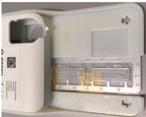
Figure 56: 3D printed cartridge used as a cell counting slide holder for optical analysis of stained cells in the Vivalytic analyzer.
