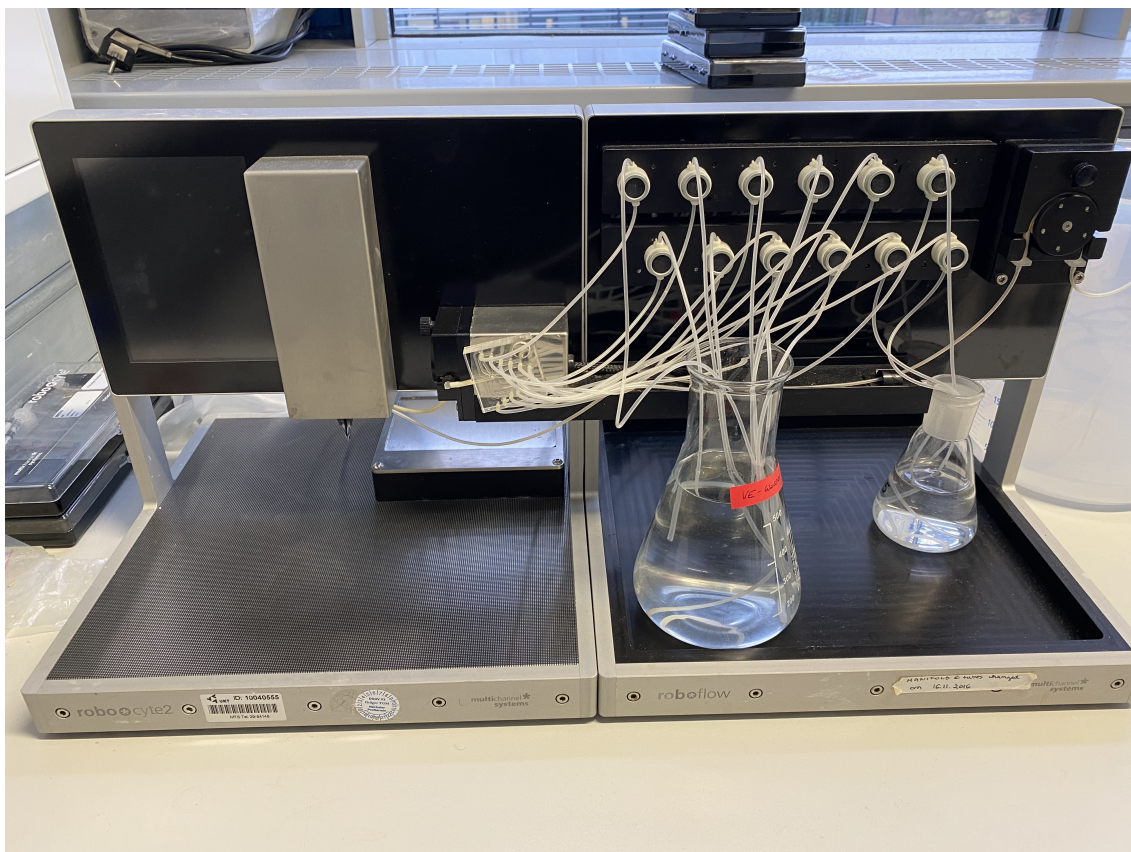
Figure 6. The fully automated Robocyte2 system as used in the experiments described (Multi Channel Systems MCS GmbH, Reutlingen).
