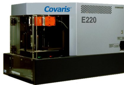
Abbildung 4: Covaris ® E220 Focused Ultrasonicator
