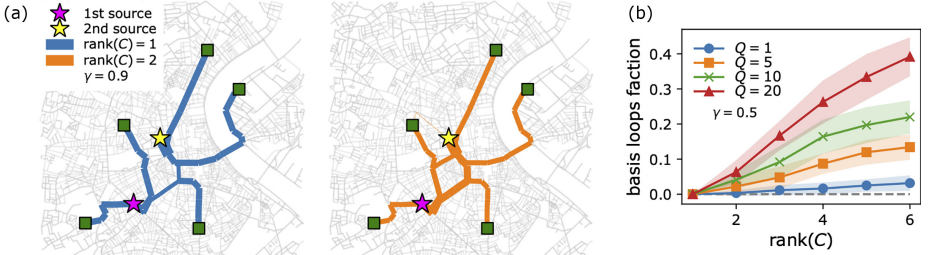
FIG. 4. Bordeaux bus optimal transport network. (a) Network visualization. Input loads have been built as described in Sec. VB. The tree network originated by C with rank 1 is plotted in blue, the loopy topology in orange. The yellow and the magenta stars denote the geographical location of the two loads, the green squares those of the sinks. Here the width of edges corresponds to slow conductivities at convergence \bar{\mu}_e^\infty . Results are plotted for \gamma = 0.9 . (b) Basis loop fraction against rank( C ). Points correspond to averages over 100 runs of the experiments where positions of the sources and sinks are extracted at random. Shaded regions denote their standard deviations. Results are displayed for \gamma = 0.5 .
