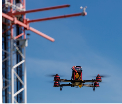
Figure 1.3: Picture of the quadrotor ‘HolyBro QAV250’ in front of the meteorological mast at Falkenberg. Photo by Bernd Lammel. This picture and description are taken from Wetz et al. (2021).
