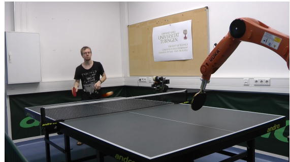
Fig. 1. Spin Detection used to return balls with high rotation on a real robot. Supplementary Video: https://youtu.be/SjE1PtU0bTo
