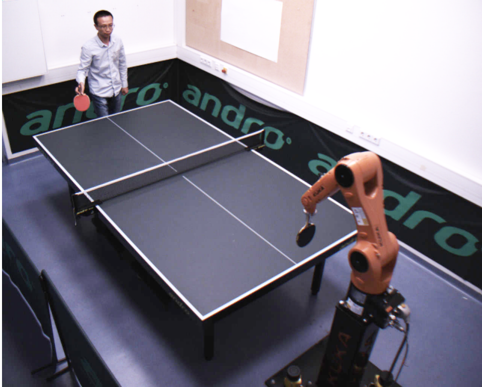
Fig. 1. Table tennis robot system with KUKA Agilus robot. There are four PointGrey Chameleon3 cameras mounted on the ceiling corners far away from each other to occupy more scenario, where two cameras opposite to human are used to detect the racket and another pair is for table tennis ball detection. A table tennis racket is rigidly fixed at the end effector of robot in a type of penhold grip. The robot coordinate is set as the world coordinate and the center of racket is defined as the tool coordinate center.
