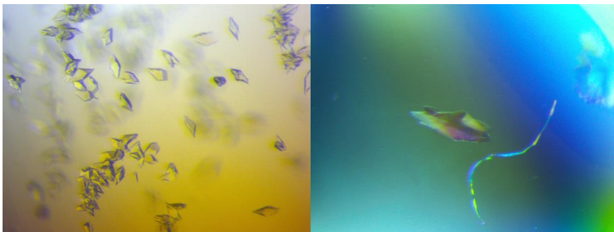
Figure 50. Image of a typical drop of DYRK1a AMP-PCP cocrystals on the left. A crystal was sent to the SLS for diffraction on the right. Crystals are typically between 0.2 and 0.3 mm in the longest dimension, with occasional larger ones up to 0.5 mm.
