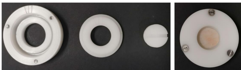
FIGURE S2 The whole setup used for confocal Raman measurements in this study. (A) unassembled three parts of the device, (B) assembled device.
